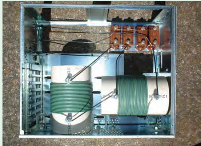
A view of the inside of the low-pass filter assembly
