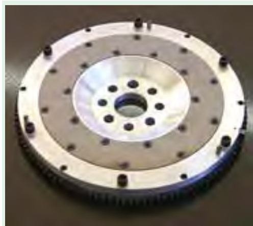
The above figure shows the flywheel of a motor as a separate part
