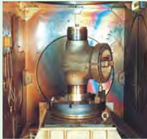
Electron beam welding facility
