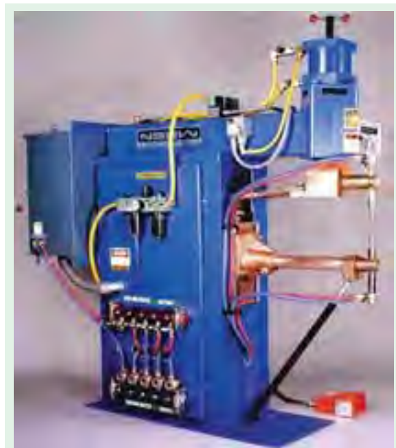
Spot welding machine
