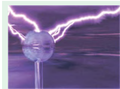
Using Van De Graff Generator, artificial lightning can be created in the laboratory, in a miniature scale.
