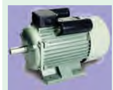
Split-phase motor. Switch mechanism disconnects start winding when motor reached three-fourths of rated speed
