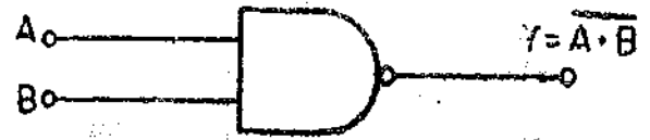
Fig. B-7. Symbolic representation of a NAND gate.
