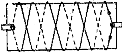
Fig. 5.6. Ayrton Perry Winding.
