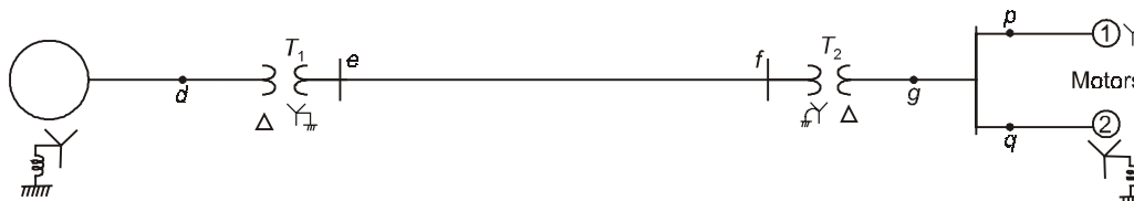
Fig. 10.11: Single-line diagram the system of Example 10.1.
