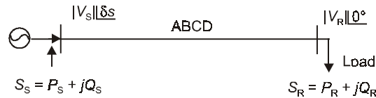
Fig. 6.7: Two bus sample power system.
